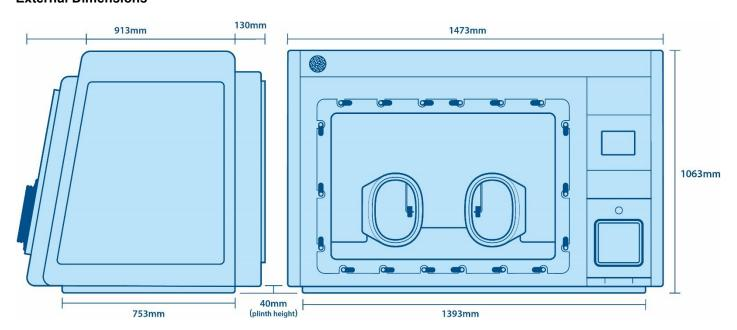
**Important note:** If bench mounted, a further minimum clearance of 500mm is required above the unit and a minimum clearance of 500mm on both sides of the unit is required for user/service access. If the **Refrigeration System** is fitted, please allow a clearance of 770mm behind the workstation. If the **Heat Removal System** is fitted, please allow a clearance of 600mm behind the workstation. Some of this clearance is necessary for air circulation.
